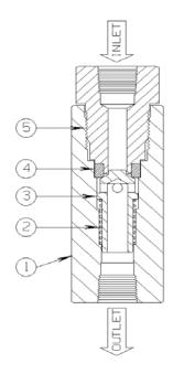
The **14KS Check Valve** is a two position, spring biased poppet operated flow control device that permits Inlet to Outlet flow only. Our Check or Flow Safety Valve (FSV) prevents reverse pressure flow from Outlet to Inlet, through spring assisted poppet positioning.
